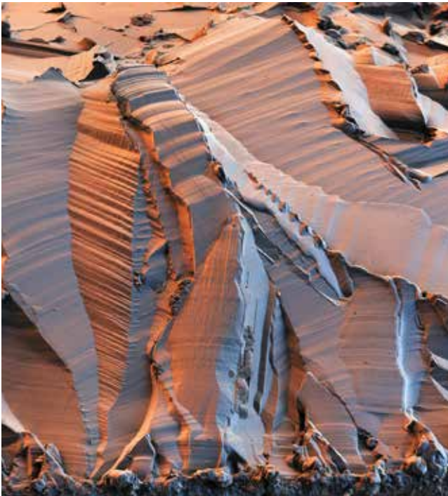
Legend: Sodium nitrate of the highest purity: In solar thermal power plants, this melted salt from BASF stores the sun's energy, which can be converted into electrical energy when needed. © BASF
